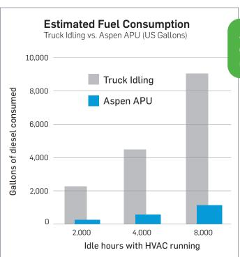
Truck idling fuel consumption –  $1.15 \text{ gph}^1$ Diesel APU fuel consumption –  $0.15 \text{ gph}^2$  At \$4 a gallon for diesel, use of an APU can generate savings of \$16,000 in reduced fuel usage after only 4,000 hours of use.
