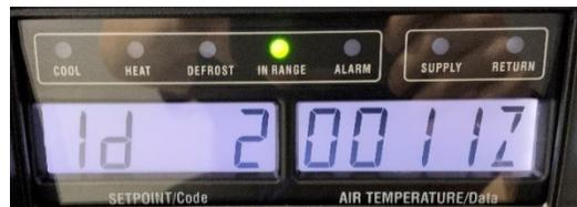
After selecting the container or entering the container ID, the password is found by pressing the ALT. MODE key, using the arrow keys to display “nEt”, and pressing the ENTER key. Use the arrows keys to display “PASSW EntR”, then press the ENTER key. The display will show a six-character password required to connect to this unit’s controller. If a five-character password is found, upgrade to SW 6315 or greater to connect via Wi-Fi.
