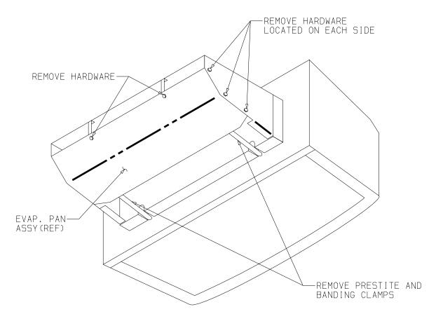
1.) REMOVE EVAPORATOR DRAIN PAN ASSEMBLY FROM UNIT(RETAIN HARDWARE FOR RE-ASSEMBLY).
