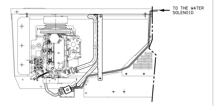
23.) ROUTE THE WATER HARNESS TO THE WATER SOLENOID. MAKE CERTAIN THAT THE HARNESS CANNOT COME IN CONTACT WITH THE CONDENSER FAN.
