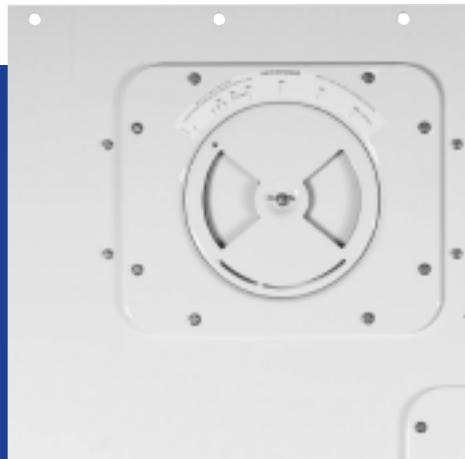
Carrier includes standard Fresh Air Exchange by an upper access panel on every NT unit to meet perishable cargo fresh air exchange needs. In addition to the standard panel, there are a number of options available to better tailor the fresh air exchange feature to the specific demands of the operation or trade. All options are compliant with the ATO fresh-air exchange requirement, which calls for an exchange rate of 2.6m<sup>3</sup>/hr/m<sup>3</sup> of internal volume.
