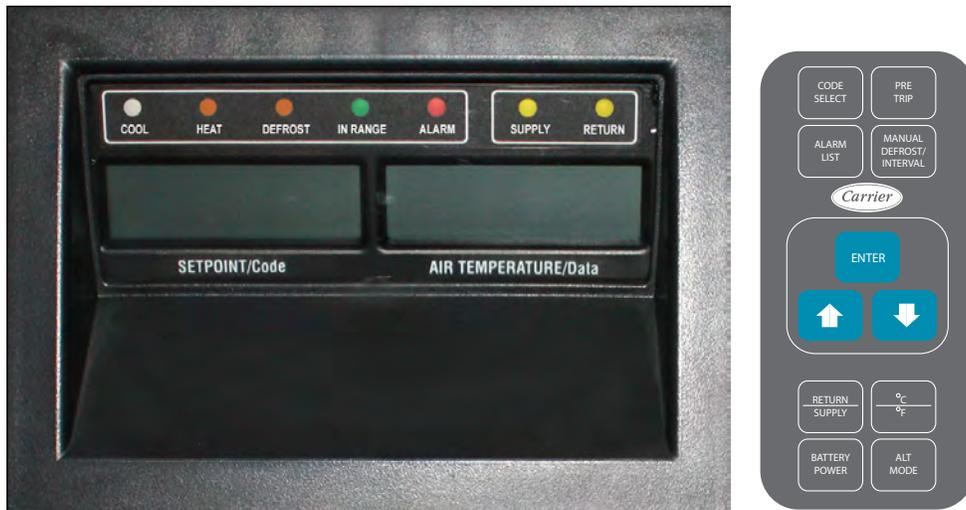
The display module consists of two 5-digit displays and seven indicator lights. The indicator lights are described in [Table 4-1](#). The keypad consists of eleven push button switches that act as the user's interface with the controller. The switch functions are described in [Table 4-2](#).
