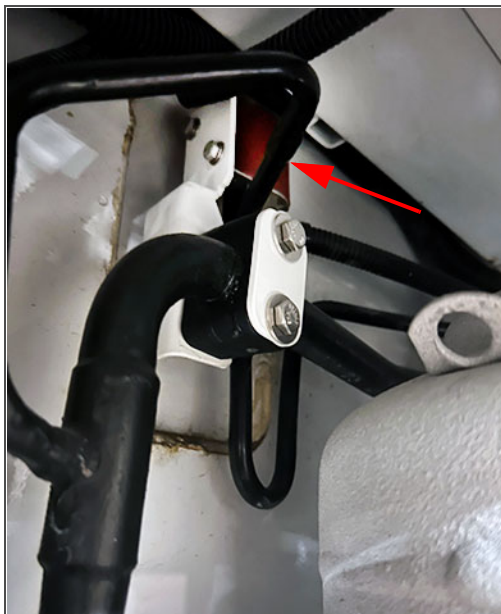
Figure 3.21 Digital Loader Valve (DLV)
