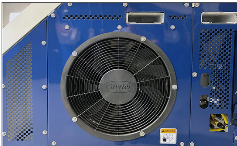
Figure 3.9 Condenser Coil and Fan
