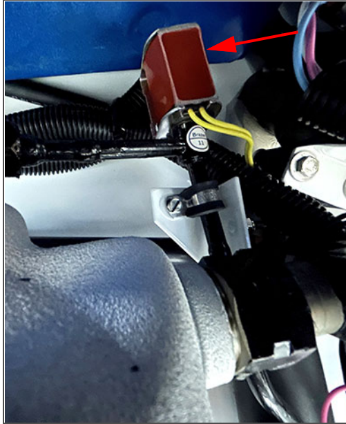
Figure 3.20 Digital Unloader Valve (DUV)
