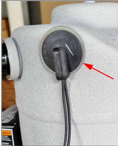
Figure 3.24 Compressor Discharge Temperature Sensor (CPDS)
