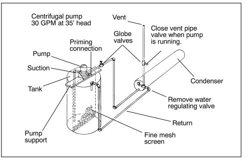
5. Allow the Oakite No. 32 solution to soak in the tube coils for several hours, periodically pump-circulating it with an acid-proof pump.
