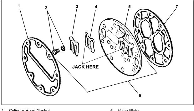
Figure 7.7 Exploded View of Valve Plate
