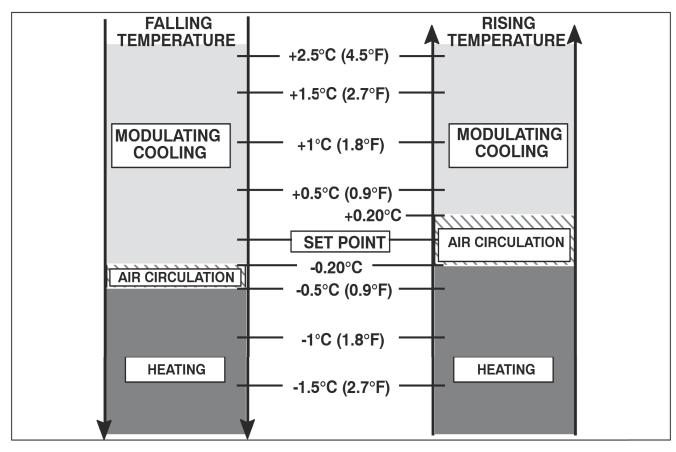
Figure 5.3 Controller Operation - Perishable Mode
