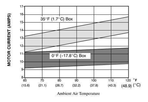
Compressor-Motor Current Versus Ambient Air Temperature At Stable Box Temperature
