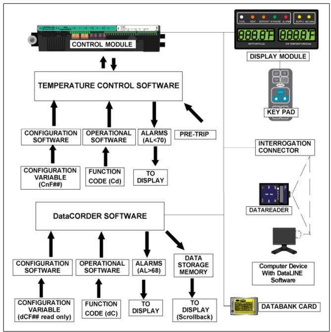
Figure 4.1 Temperature Control System
