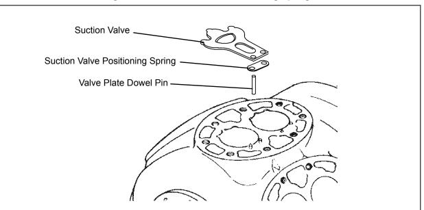
Figure 7.14 Suction Valve & Positioning Springs
