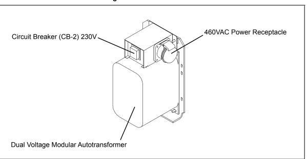
Figure 5.1 Autotransformer
