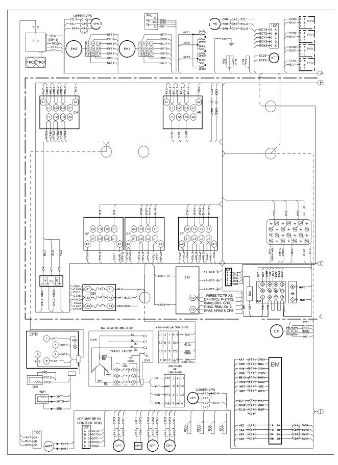
Figure 8.7 UNIT WIRING DIAGRAM (Sheet 1 of 2)
