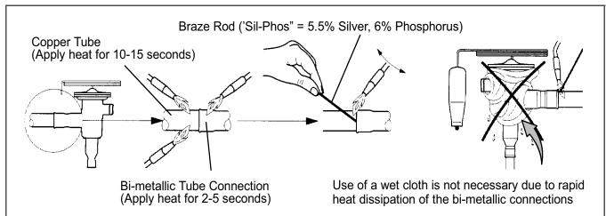
Figure 7.21 Hermetic Thermostatic Expansion Valve Brazing Procedure
