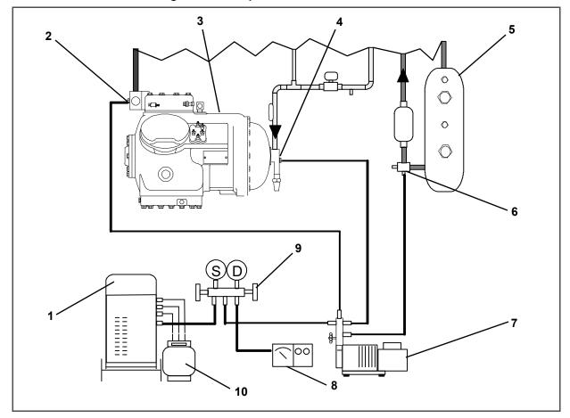
Figure 7.5 Compressor Service Connections
