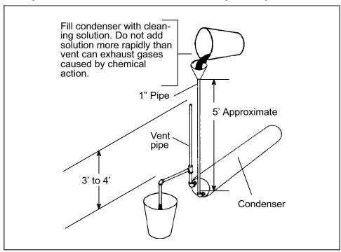
Figure 7.18 Water-cooled Condenser Cleaning - Gravity Circulation
