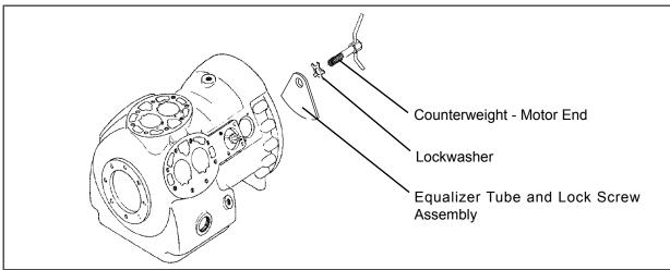
Figure 7.12 Equalizing Tube and Lock Screw Assembly
