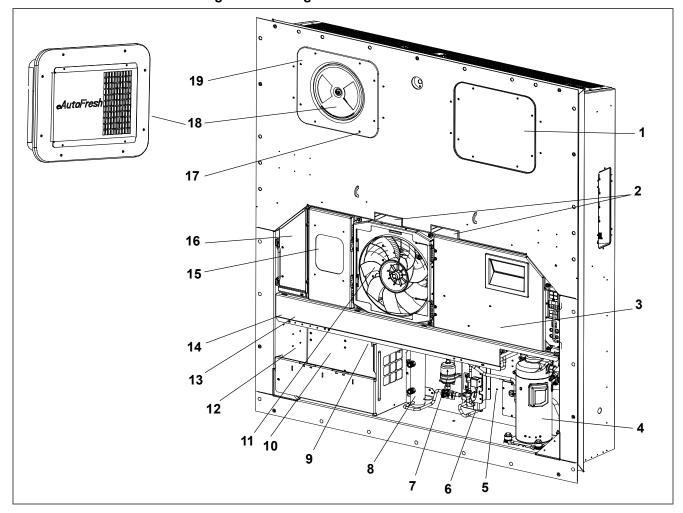
Figure 3.1 Refrigeration Unit - Front Section
