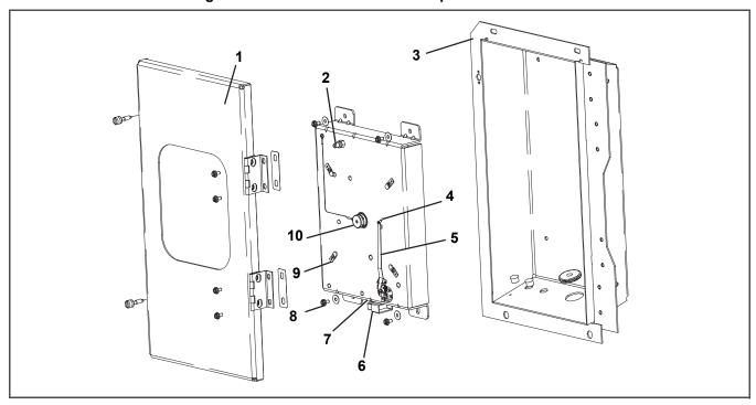
Figure 7.37 Electronic Partlow Temperature Recorder
