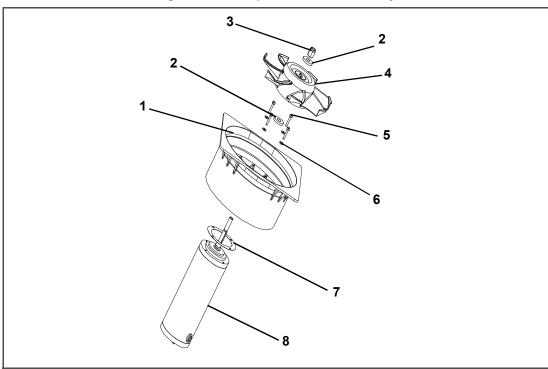
Figure 7.10 Evaporator Fan Assembly
