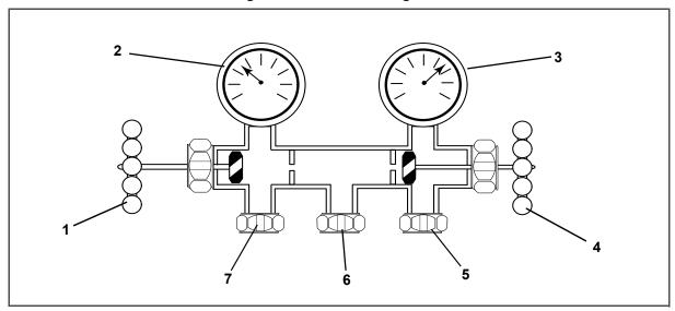
Figure 7.1 Manifold Gauge Set
