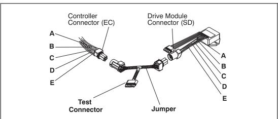
Figure 7.35 Jumper Assembly
