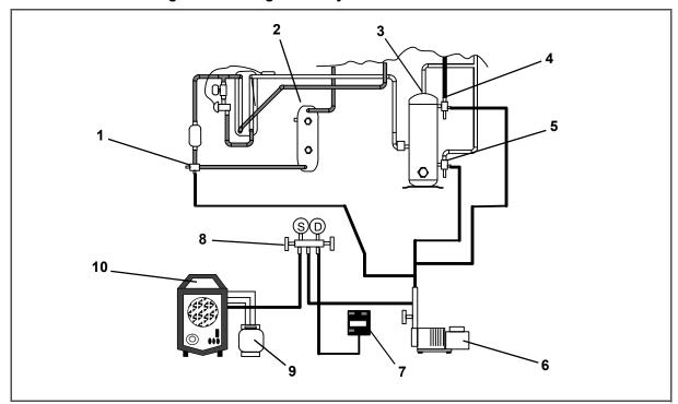
Figure 7.4 Refrigeration System Service Connections
