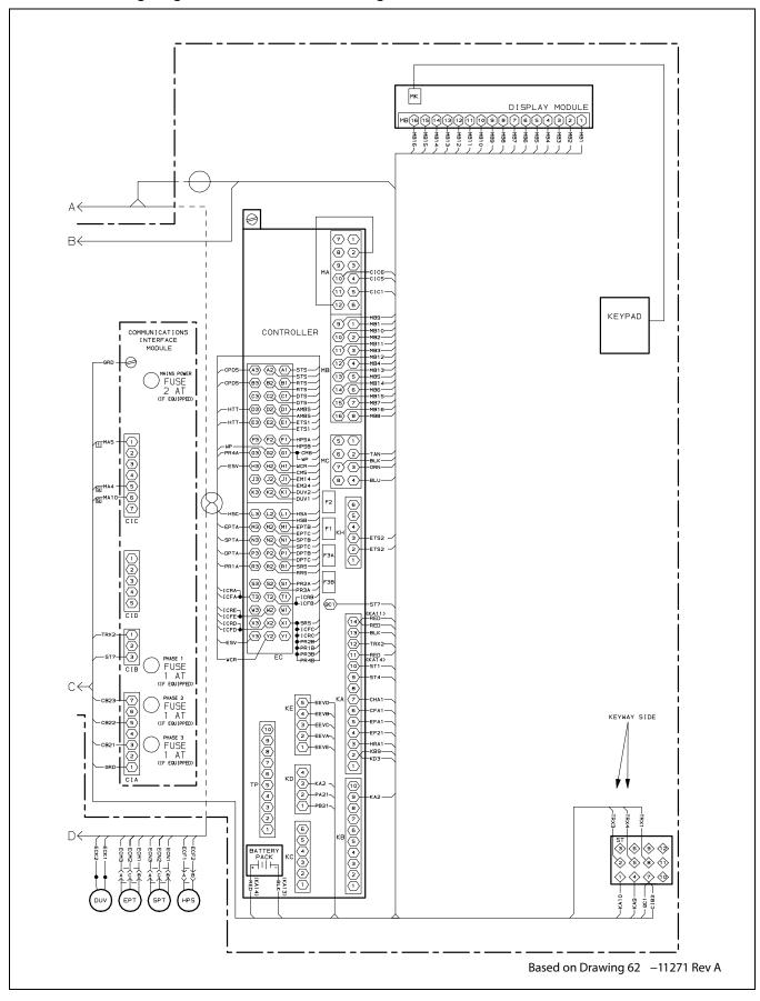
Figure 8.10 Unit Wiring Diagram for Single Phase Condenser Fan Motor and Optional Heater
