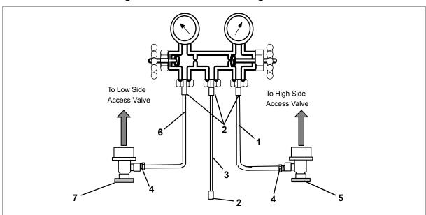
Figure 7.2 R-134a Manifold Gauge/Hose Set
