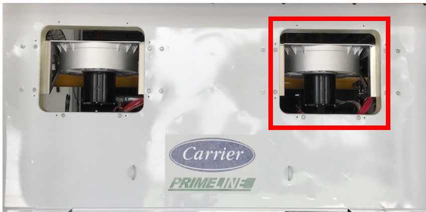
Figure 7.27 Removing Evaporator Motor
