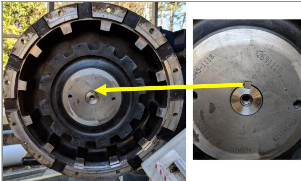
20. Apply Loctite 262 to the generator coupler bolt. Install with washer and torque to 28 ft-lbs (38 N-m). See [Figure 5.7](#).
