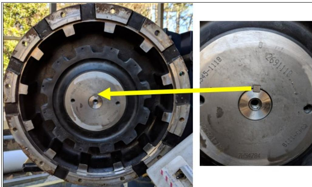
20. Apply Loctite 262 to the generator coupler bolt. Install with washer and torque to 38 N·m (28 ft-lbs). See [Figure 5.7](#).
