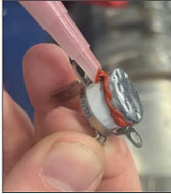
7. Position the switch over the holes with the rim flat to the body of the DOC.
