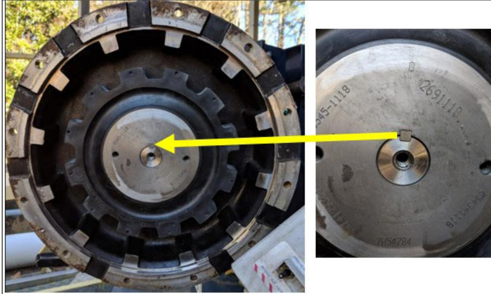
20. Apply Loctite 262 to the generator coupler bolt. Install with washer and torque to 28 ft-lbs (38 Nm). See [Figure 6.2](#).
