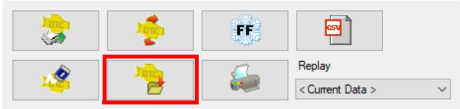
2. A pop up screen appears. A memo can be added prior to saving. The file name for the saved data is automatically chosen. Click the Save button to complete the save.
