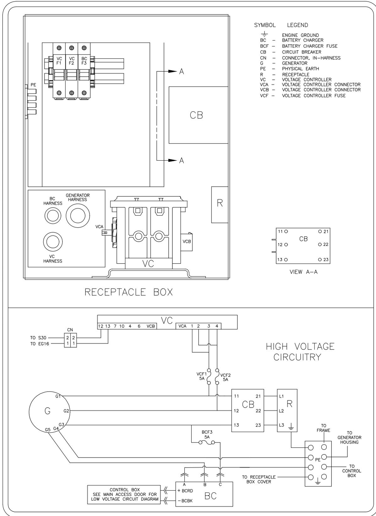
**Figure 8.4 Schematic High Voltage Circuitry (PID UG2403 only)**
