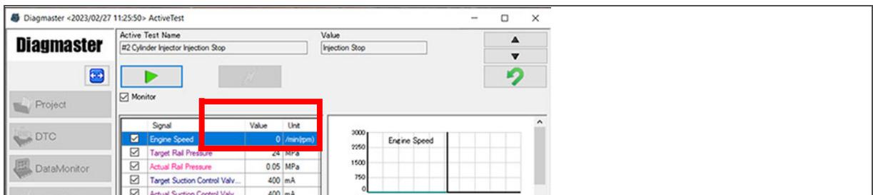
4. Click the yellow button to execute the active test. Driving instructions will be sent to the ECU. Check the operating noise of the actuator. During the active test, flags can be added by clicking the flag button.
