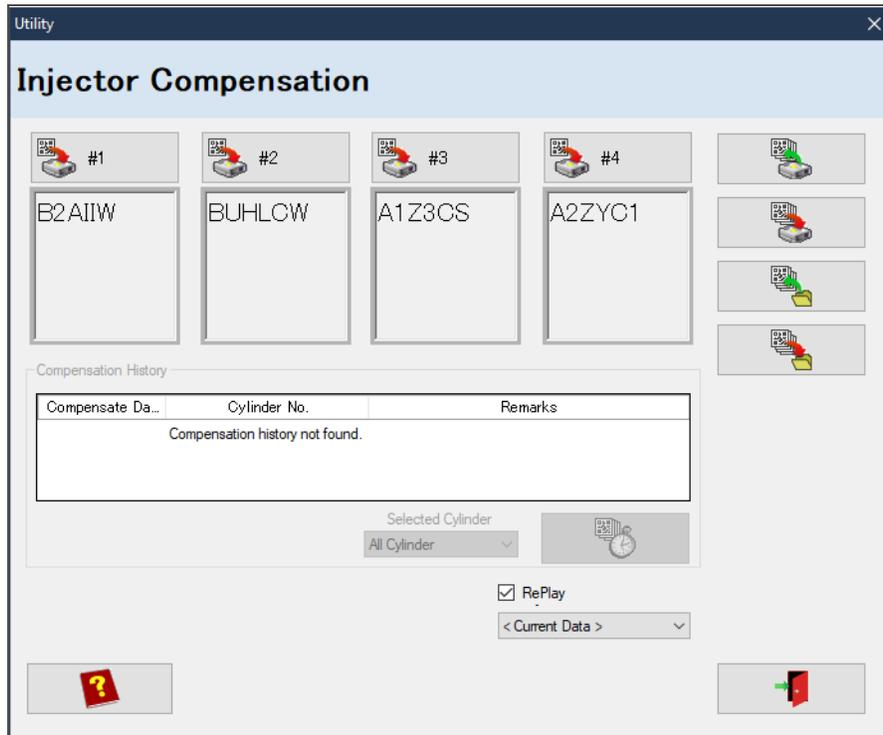
2. Click on any register individual injector button. Or, click on the register all injectors button to register all injectors at once.
