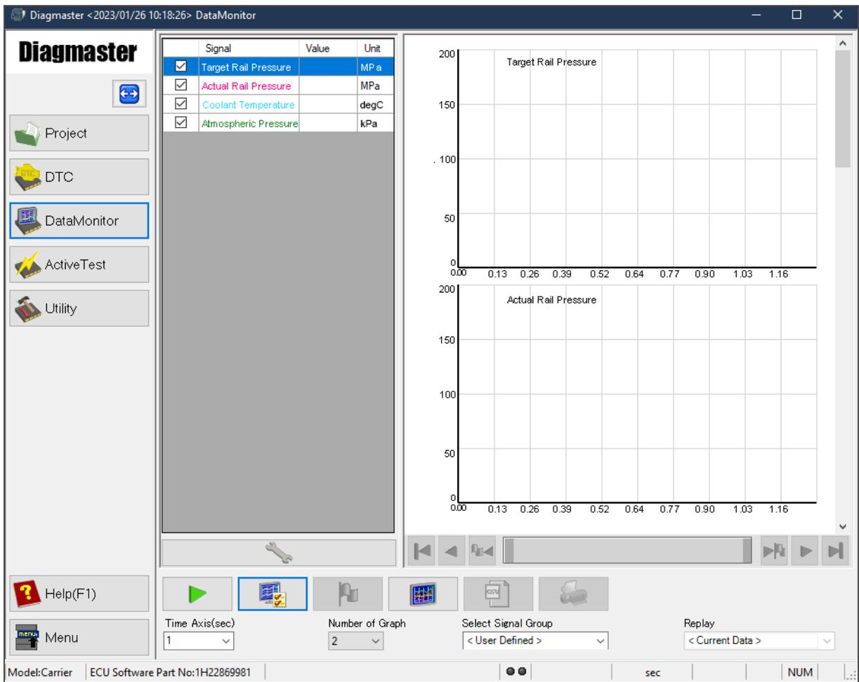
9. Signal settings that have been previously saved are stored in the Select Signal Group drop down box and can offer a way to store favorite settings for quick access.
