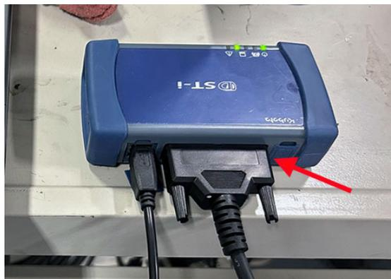
3. Locate the Kubota Service Port (KSP) on the unit. Remove the dust cap.
