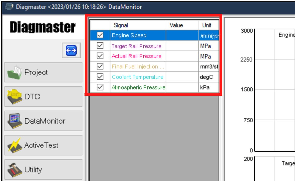
6. Click the Play button (green) to start data measurement and Stop button (gray) to finish. During a measurement, observe the data on screen when the engine is stopped (ignition RUN) and also when the engine cranking (ignition START). Check the measurements for each of the settings active in the screen and compare to the reference values given in the tables below.
