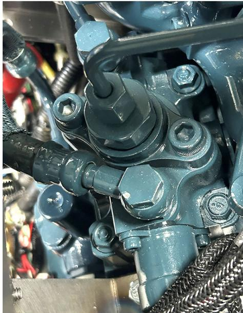
The engine side fuel camshaft rotates and during the lowering stroke a spring causes the plunger to lower. An optimal amount of fuel adjusted by the suction control valve (SCV) is suctioned through the IO valve and into the plunger chamber. During the lift stroke of the cam the plunger rises, which pressurizes the fuel and supplies it through the IO valve to the rail.
