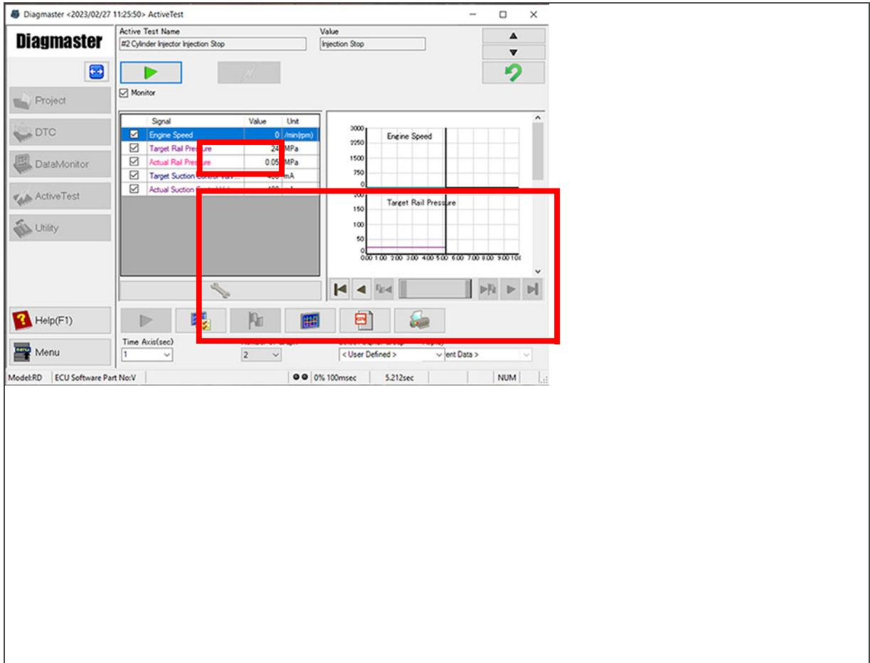
3. Click the green play button to make active tests ready to be executed. Data monitoring will start if simultaneous monitoring has been selected.
