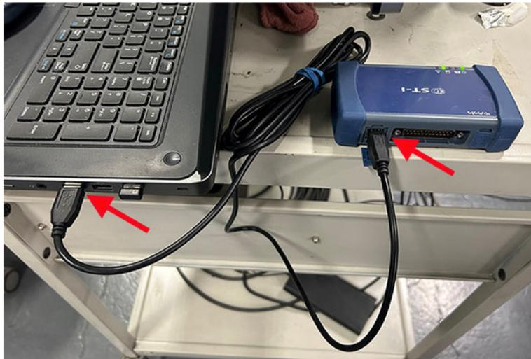
2. Connect one end of the data link cable to the DST-i device.
