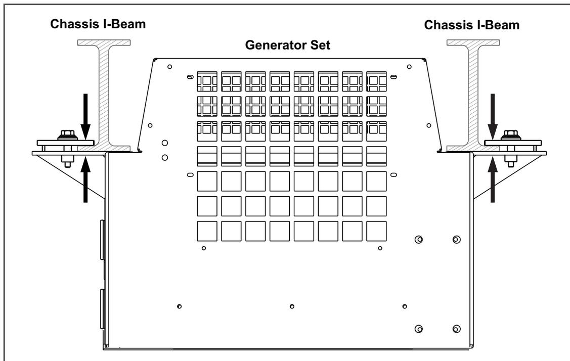
6. Slide the mounting plates fully onto the chassis I-beams and torque mounting bolts to a minimum of 200 ft-lbs (271 Nm), in a cross pattern. The torque range is 200 to 260 ft-lbs. (271 to 352 Nm).
