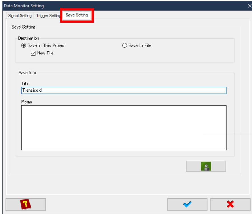
7. When finished with all data monitor settings, click the blue checkmark to complete and close the window.
