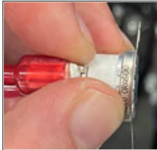
8. Attach the switches to the DOC using 4 stainless steel rivets and a powered rivet tool to ensure tightness of installation. Ensure the bracket is flat against the switch head.
