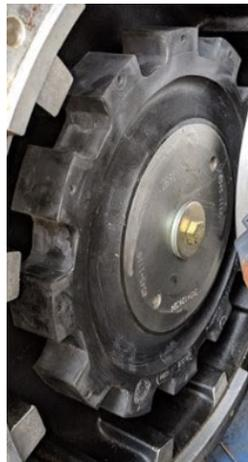
**NOTE:** In order to torque generator torsional dampener gear bolt, use a strap wrench or similar device to secure the dampener while torquing the bolt.
