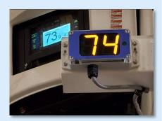
Union Pacific's refrigeration system specifications for its new boxcars include a bright external LED temperature display (above) and a TRU-mount solar panel to charge the Vector unit battery, which also supports telematics functions. An ultrasonic sensor in the 435-gallon fuel tank and a differential fuel flow meter enable diesel fuel levels and consumption to be remotely monitored and analyzed.
