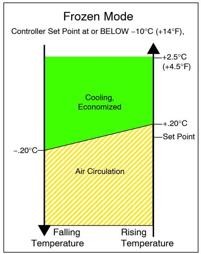
Figure 3-8 Controller Operation - Frozen Mode
