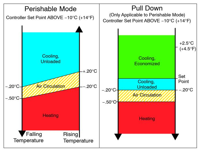
Figure 3-5 Controller Operation - Perishable Mode
