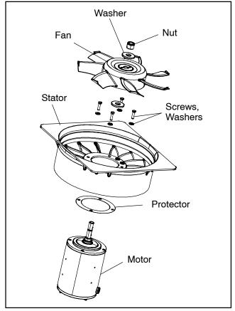
Figure 6-8 Evaporator Fan Assembly
