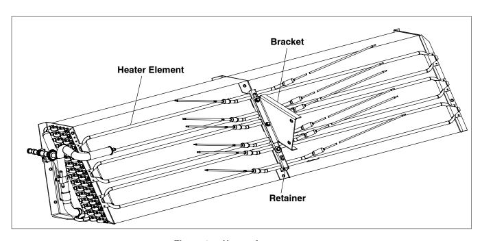
Figure 6-7 Heater Arrangement
