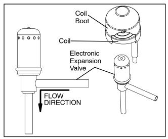
Figure 6-9 Electronic Expansion Valve
