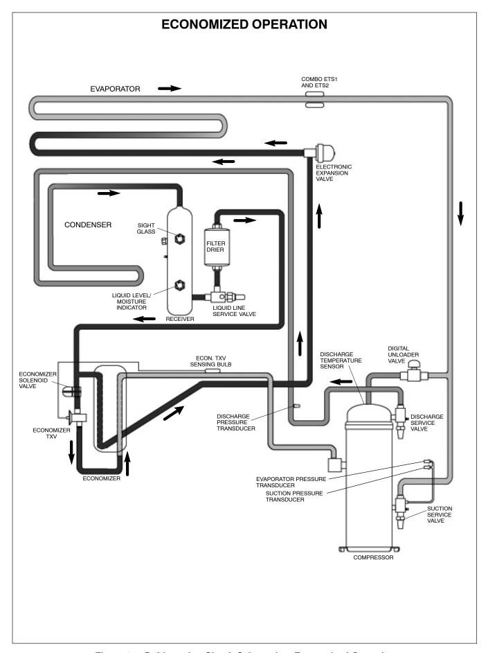
Figure 2-7 Refrigeration Circuit Schematic - Economized Operation
