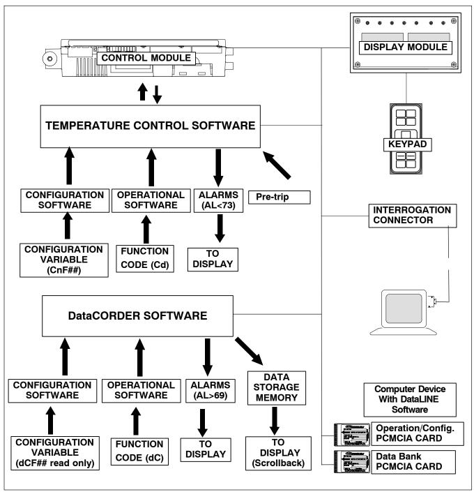
Figure 3-1 Temperature Control System
