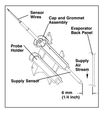
Figure 6-16 Supply Sensor Positioning
