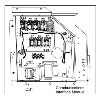
Figure 6–20 Communications Interface Installation
