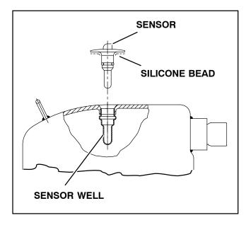
Figure 6–19 Compressor Discharge Temperature Sensor
