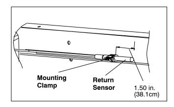
Figure 6-17 Return Sensor Positioning
