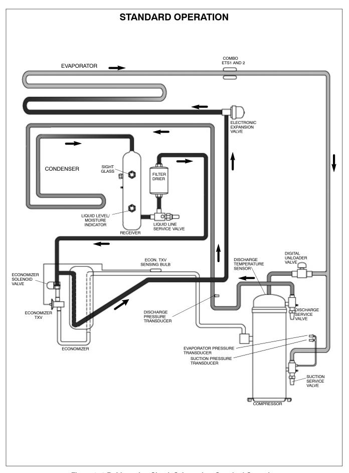
Figure 2-6 Refrigeration Circuit Schematic - Standard Operation
