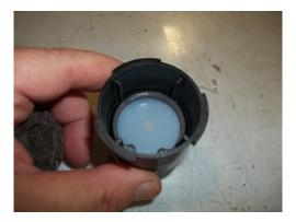
4. Install the new felt filter and then replace the filter cap by pressing up into the slot and turn a 1/4 turn clockwise to lock.
