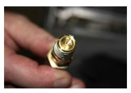
6. Reverse the above steps to re-install the orifices. The orifice end of the connector faces away from the Tee when being re-installed.
