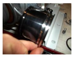
2. Install the black ring over the silver ring on the piston. Open slightly to get over the piston and slide into place. Offset the ring gap by 180 degrees.
