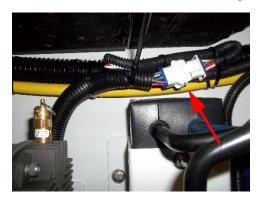
3. Using a 5/8" wrench, remove the air compressor discharge line.
