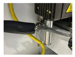
5. Using a 9/16" socket, remove the four mounting bolts from the compressor and six bolts securing the front bracket.
