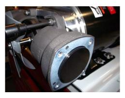
6. Remove the piston guide and rings from the piston.
