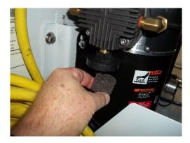
3. Clean any debris out of the filter housing.
