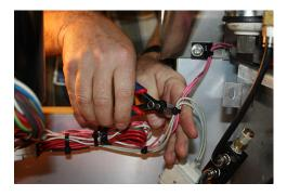
10. Disconnect the WDV by turning it with a 3/4" wrench and using a 9/16" wrench to hold the mating connector.
