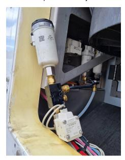
7. Remove the Water Drain Valve (WDV) from the manifold. Check the inlet for any debris and, if present, collect a sample. Blow out the WDV with shop air and set aside to reinstall after the Water Separator is inspected.
