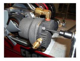
4. Remove crossbars from the air compressor using a 3/4" wrench.
