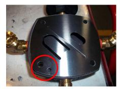
6. Install the new valve plate by aligning the indicator hole on the plate to the discharge valve. When properly installed, two holes will cover the discharge valve and two holes the head is visible. If you cannot see the head on two adjacent holes, the backer plate is not installed properly.
