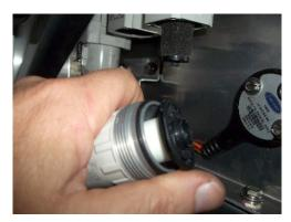
7. Then install the housing back onto the filter body by rotating clockwise until snug.
