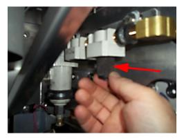
4. Remove the second filter from the filter housing by pressing up on the locking tab holding the filter in place.
