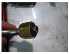
10. On the second head, repeat steps 4 through 8. When installing heads in step 8, ensure crossover pipes are properly seated into the head fittings prior to torquing head bolts. Tighten the crossover compression nuts. Re-torque the cylinder heads to 150 to 160 in-lbs. (17 to 18 Nm).
