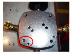
7. Lay the gasket without material in the center on the backer plate. Align the two indicator holes.
