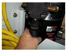
2. Remove the felt filter.
