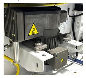
2. Install the remaining four pieces of metal cushions + four pieces of cushion seats as shown and align to the holes on the bracket. Tighten the compressor to the bracket with the four saved 2.25" long screws using a 9/16" socket.
