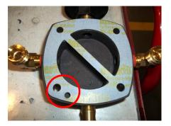
5. Take the outlet valve plate with the line down the center and align with the indicator hole.
