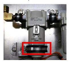
5. Pull down the locking clamp and turn a 1/4 turn clockwise, and drop the Water Separator bowl.
