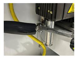
6. Reattach the shield with the four saved 3/4" long screws using a 1/4" socket. Torque to 3.05 Nm / 27 in-lbs.
