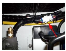
3. Using a 1/4 socket, remove the shield from the left of the compressor.
