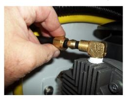
4. Connect the air compressor power connection and wire tie the harness to the drain line and yellow power cable. Maintain a drip loop on the power line prior to entering the compressor motor.
