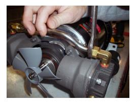
3. Remove the head with loosened crossbar nuts using a 3/16" hex key. Remove the four head bolts and pull off the head assembly including valve plates. Discard bolts, do not reuse.
