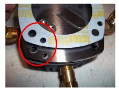
8. Place head bolts into two of the holes to maintain alignment of the gaskets and plates and install the head onto the cylinder. Hand tighten the four head bolts. Then rotate the crankshaft to verify the piston does not hit the head. If it doesn't hit, torque the head bolts to 150 to 160 in-lbs. (17 to 18 Nm) and recheck. If the head does hit, return to step 3 and realign the cylinder.
