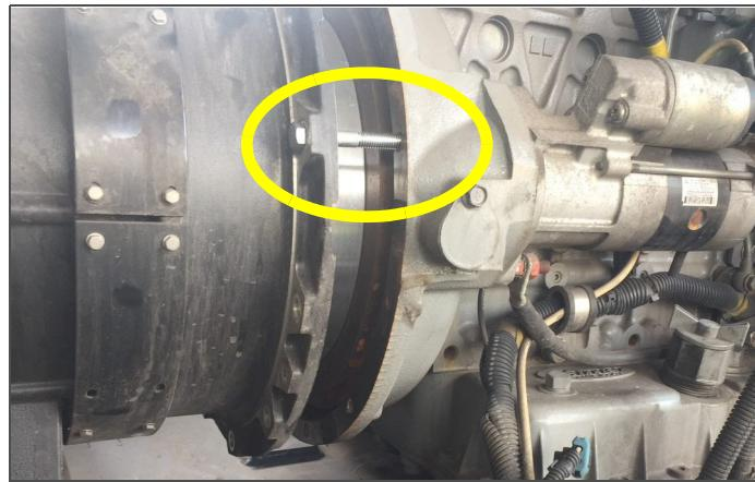
24. Once aligned, push the generator to fully seat the torsional dampener into the aluminum housing of the flywheel adaptor plate.
