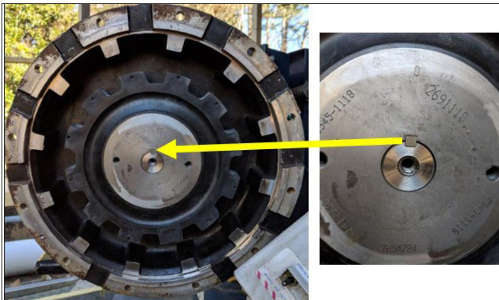
20. Apply Loctite 262 to the generator coupler bolt. Install with washer and torque to 28 ft-lbs (38 Nm). See [Figure 6.6](#).
