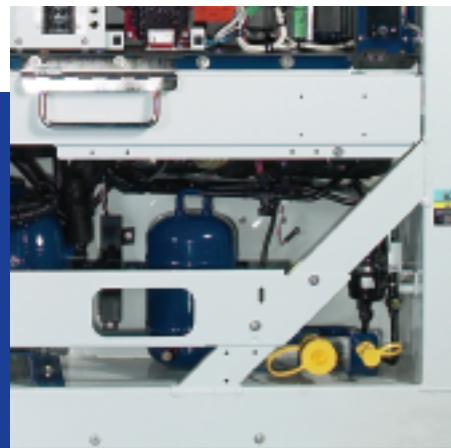
To reduce heat buildup in the ship's hold, Carrier units may be ordered with an optional Carrier-manufactured water-cooled condenser, which delivers condensing performance equivalent to air-cooled operation in 38° C (100° F) air temperatures with water temperature of 30° C (86° F) and flow of .38 L/s (6 gpm).
