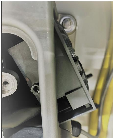
8. The replacement fan (part # 10-00560-31) comes with new wire grommet installed. Assemble the replacement VFD fan by reversing the order of the above steps:
