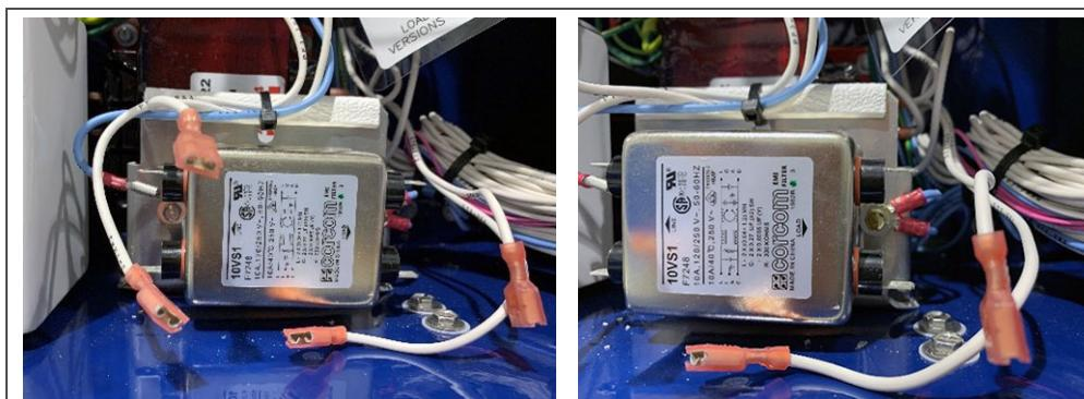
3. Remove the remaining mounting bolt on the left side (line input) and pull from the system control box.
