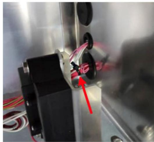
16. On the right side of the fan deck, bundle the wires with cable ties.
