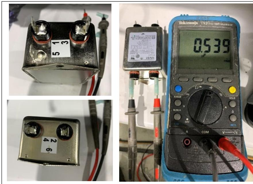
5. Each individual pin can also be verified between the ground pin #5 and 1, 2, 3, 4. Testing each individual pin to the ground pin should read a capacitance of 0.011 uF +/-10%. Note that meter to left reading in nF but passing value 0.01052 uF.
