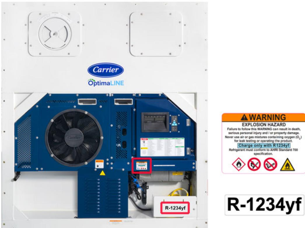
13. Install the fire warning label (p/n 62-66268-00) on the upper back panel and the container rear door. Install the flammable warning labels (p/n 62-12442-00 and 62-12444-00) on the container rear door.
