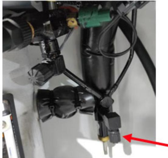
6. Apply lubricant (p/n 46-00058-00) on the o-ring of the low side charge port (p/n 40-00812-00). Replace the current charge port with the new charge port. Use 2 wrenches and tighten to 114 lbf-in.
