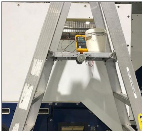
7. Once temperature stability is ensured, submerge the sensors in the ice water slurry. Make certain that the sensors do not contact the container sides or bottom, or each other. Continuously stir the slurry mixture during calibration.
