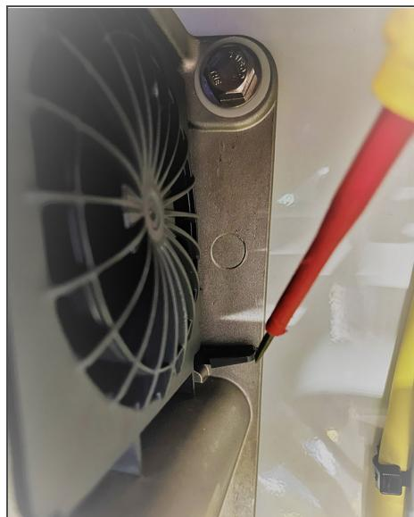
7. Pull the lower end of the fan assembly radially out. Use a screwdriver to pull out the fan assembly if needed.
