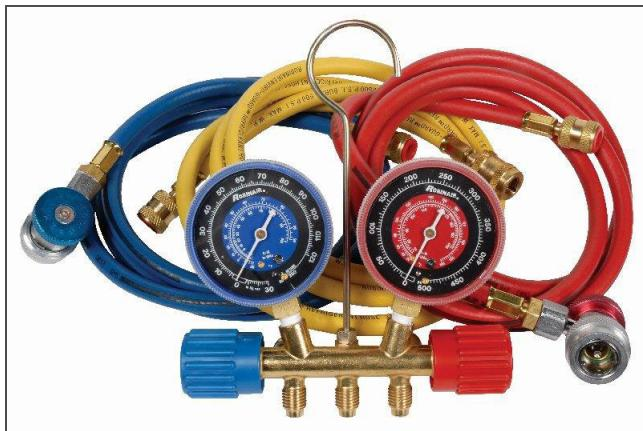
The gauge set layout with hoses and couplings is shown in **Figure 7.2**. The gauge set connects to the service connections on the refrigeration unit using the blue and red hoses. Service connections are described in **Section 7.1.3**. The yellow hose is a utility connection that can be connected to a a refrigerant cylinder or vacuum pump.
