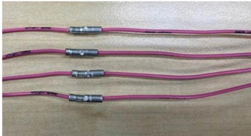
13. Move the heat shrink over the butt splice and heat shrink the wires using a heat shrink gun.
