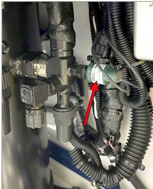
Figure 3.23 Pressostat haute pression (HPS)
