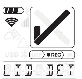
The image shows a SmartMonitor display with various status icons at the top: battery level, Wi-Fi signal, cellular signal strength, and a cloud with a checkmark. Below these is a USB icon and a control bar with 'OFF' and 'REC' buttons. The main display area shows the text 'LID DET' in a large, segmented font. | <p>Short press the multifunctional button to cycle through the menu items until the <b>LID DETECTION RESET</b> option appears.</p> |
