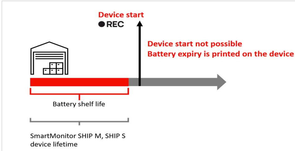
If the device is not started within battery shelf life, the battery expires. The device can no longer be started. Devices can be returned to Sensitech for recycling and refurbishment.
