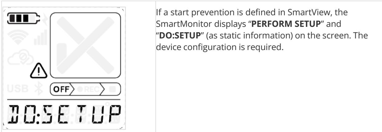
After completing the setup in SmartView, a **triple push of the multifunctional button** is required to synchronize configuration policy. After successful synchronization, the SmartMonitor can be started.
