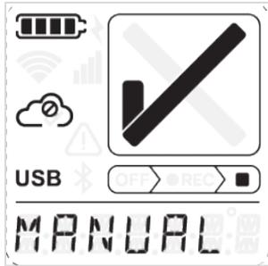
Device indicates that manual transfer of monitoring data to SmartView is required. Review SmartView manual to find out how to upload the monitoring data to SmartView.
