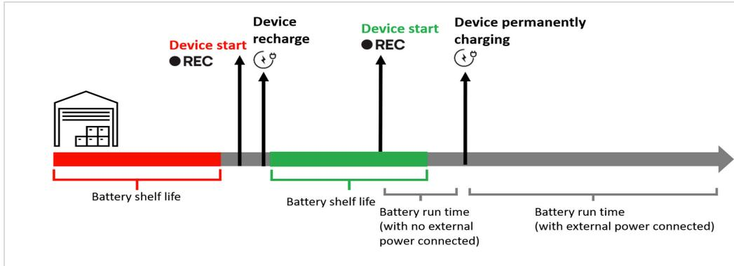
If the device is not started within battery shelf life, recharge is required to ensure battery performance according to the product data sheet.
