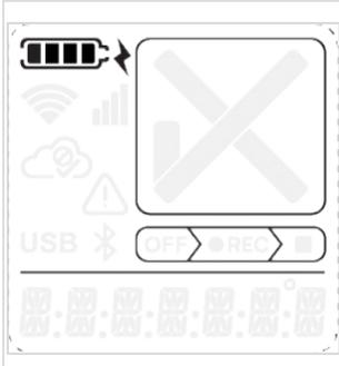
The device is connected to power and fully charged.
