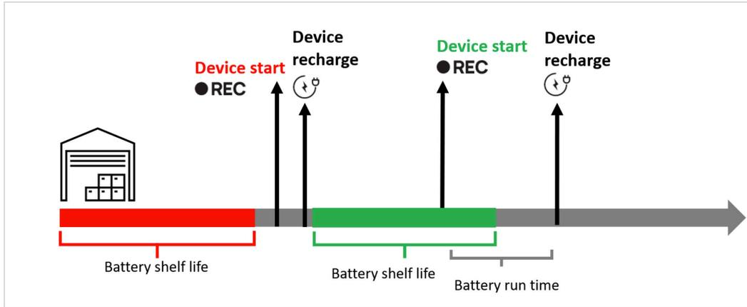
If the device is not started within battery shelf life, recharge is required to ensure battery performance according to the product data sheet.
