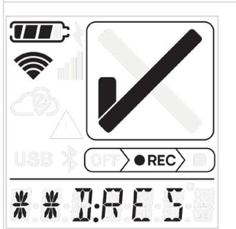
The image shows the same SmartMonitor display as above, but the main display area now shows the text 'LID:RES' in a large, segmented font.                                                                                                                                                                             | <p>To perform the reset, long press the multifunctional button. The scrolling text will display <b>LID:RES</b>.</p>                |
