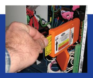
Carrier Transicold's PC Card Adapter delivers the MicroLink 3 programming ease to units equipped with MicroLink 2 (ML2) and MicroLink 2i (ML2i) controllers. So, instead of fading into obsolescence, older controllers can now benefit from the convenience of today's ML3.
