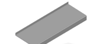
Air baffle acrylic (air guidance needed for hooks)
