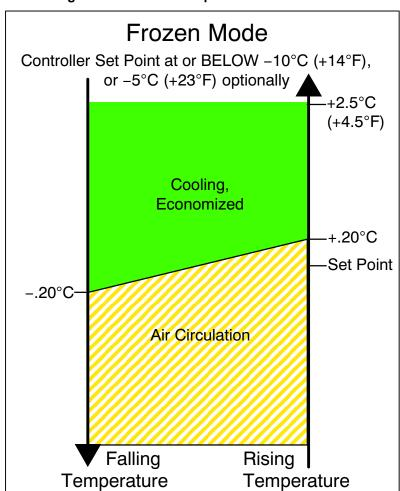
Figure 4.8 Controller Operation - Frozen Mode
