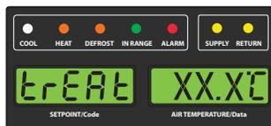
6. "dAyS" is now displayed in the left display and the right will be flashing. Use the Arrow keys to select the desired days for cold treatment and press the ENTER key.
