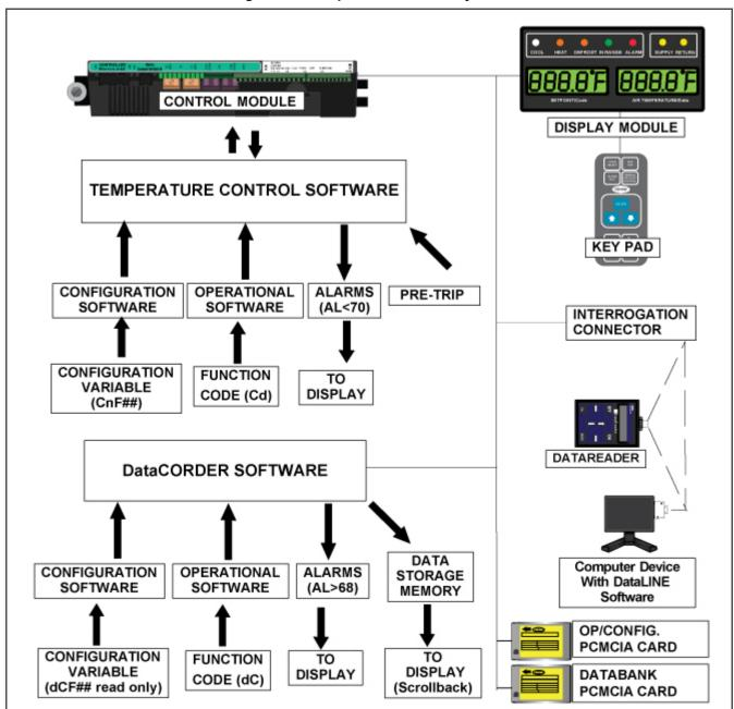
Figure 4.1 Temperature Control System
