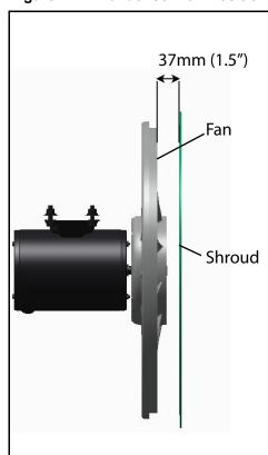
Figure 7.12 Condenser Fan Position
