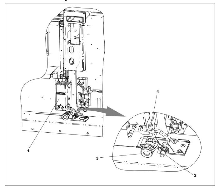
Figure 3.5 Brazed-Plate Water-Cooled Condenser
