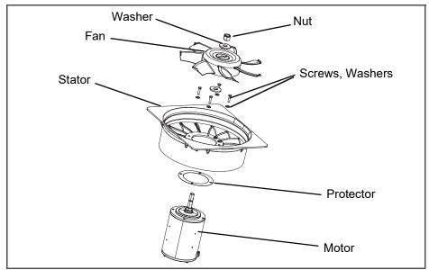
Figure 7.14 Evaporator Fan Assembly
