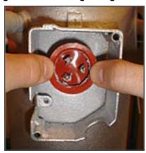
c. Coat the inside of the power plug (female) connector pins with the Krytox lubricant (Figure 7.5, item #13), and Insert the plug onto the compressor terminal connections. Make sure, the orange gasket has bottomed out onto the fusite and it fits securely onto the terminal pins while fully inserted into the orange plug as shown in Figure 7.9 and Figure 7.10.
