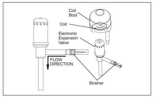
Figure 7.15 Electronic Expansion Valve
