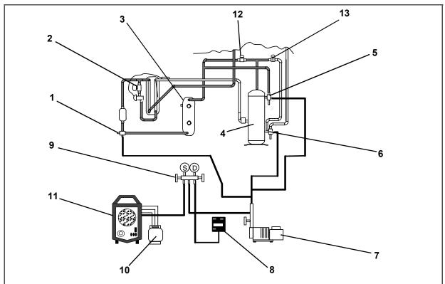
Figure 7.4 Refrigeration System Service Connections
