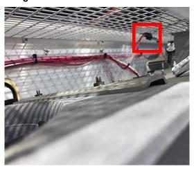
4. Cut all the wire ties (see Figure 7.26) that are securing the sensors to the harness and remove sensor.
