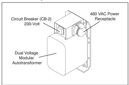
Figure 7.20 Autotransformer
