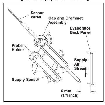
Figure 7.35 Supply Sensor Positioning
