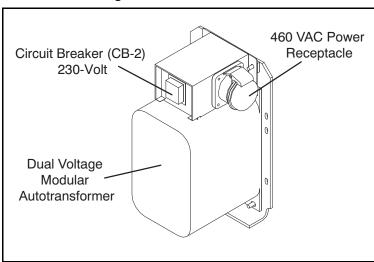
Figure 5.1 Autotransformer
