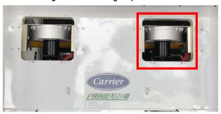
3. Loosen the fastener on the sensor bracket (see Figure 7.25).
