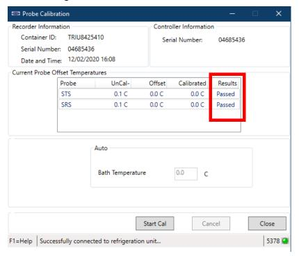
11. After completing the calibration event, download a DCX file and check that all of the following information is captured: service center name, location, the results of the calibration and the offset applied. Ensure that all the information is captured and the event is considered a success when all the intended sensors in calibration have passed.
