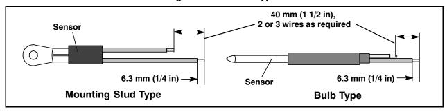
6. Slide a large piece of heat shrink tubing over the cable, and place the two small pieces of heat shrink tubing, one over each wire, before adding crimp fittings as shown in **Figure 7.34**.
