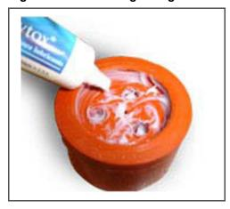
b. Install the orange gasket part onto the compressor fusite with the grooved or threaded side out as shown in **Figure 7.8**. Ensure that the gasket is seated onto the fusite base.
