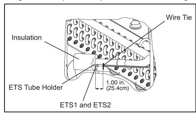
Figure 7.37 Evaporator Temperature Sensor Positioning
