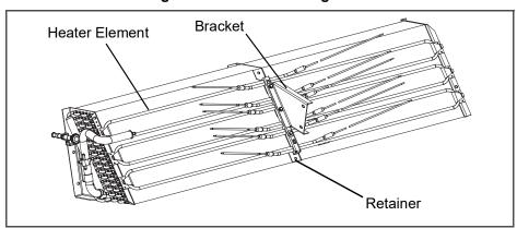
Figure 7.13 Heater Arrangement
