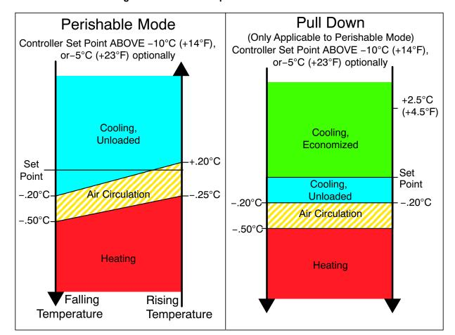
Figure 4.5 Controller Operation - Perishable Mode
