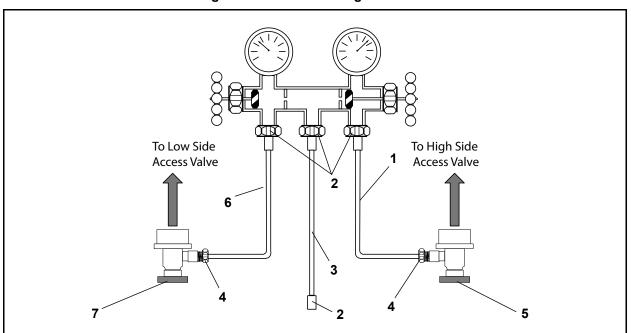
Figure 7.2 Manifold Gauge/Hose Set
