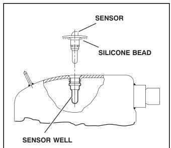
Figure 7.38 Compressor Discharge Temperature Sensor
