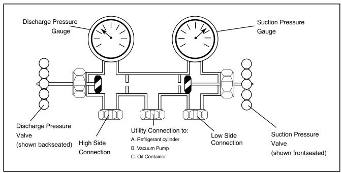
Figure 7.1 Manifold Gauge Set
