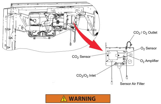
Potential hazardous atmosphere and low oxygen levels inside the container, ventilate before entering. Stay away from doors while venting. Refer to Section 4.7.
