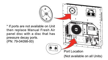
One of the ports is connected to a pressurized air supply and the other is connected to a Magnehelic pressure gauge. The pressure gauge monitors the container leakage rate.
