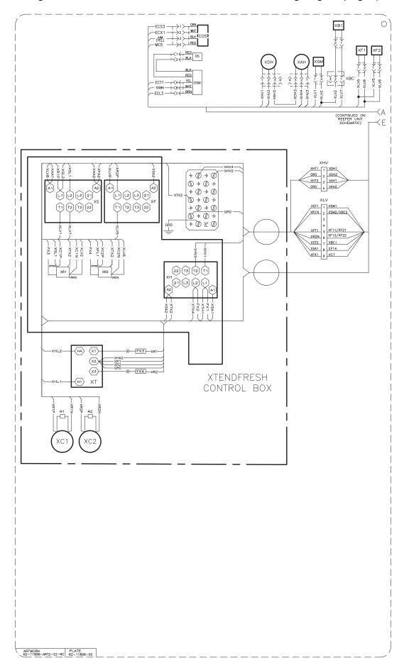
Figure 7.5 PIDs NT2570 and NT2617 - Schematic and Wiring Diagram (Page 2)
