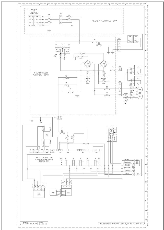
Figure 7.4 PIDs NT2570 and NT2617 - Schematic and Wiring Diagram
