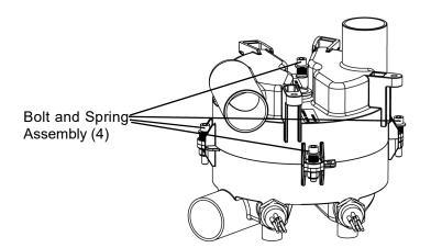
7. Separate the upper and lower halves of the scrubber housing.
