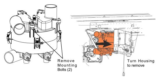
Figure 6.11 Removing the Scrubber Housing
