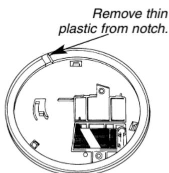
13. Position smoke alarm to mounting plate and turn clockwise to lock into place. (To engage tamper resist feature, insert pin into notch on edge of smoke alarm after smoke alarm is positioned properly in base. Refer to step #10 on previous page.)
