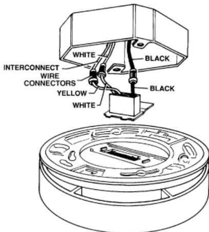
**NOTE:** If this will be a single-station smoke alarm, cover yellow wire with electrical tape and tuck into junction box.
