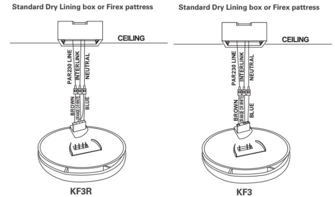
3. Using a suitably-rated terminal block, (supplied with Firex pattresses), connect the line supply to the brown lead of the connector plug.
