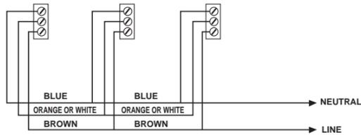
FOR INTERCONNECTING: USE A MINIMUM OF 1.5mm<sup>2</sup> CABLE
