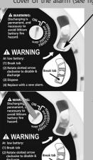
• Push in the dashed area with a screwdriver to break tab.
