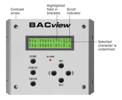
**NOTE** You can turn the contrast screw on top of the BAC*view* device clockwise to lighten the display or counterclockwise to darken it.
