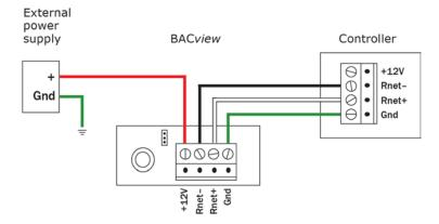
Set the address of each device by putting one device's jumper in the top position and the other's jumper in the bottom position.
