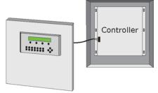
BAC*view* device mounted on panel door
