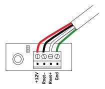
**CAUTION** Allow no more than .06 inch (1.5 mm) bare communication wire to protrude. If bare communication wire contacts a metal surface other than the terminal block, the sensor may not communicate correctly.
