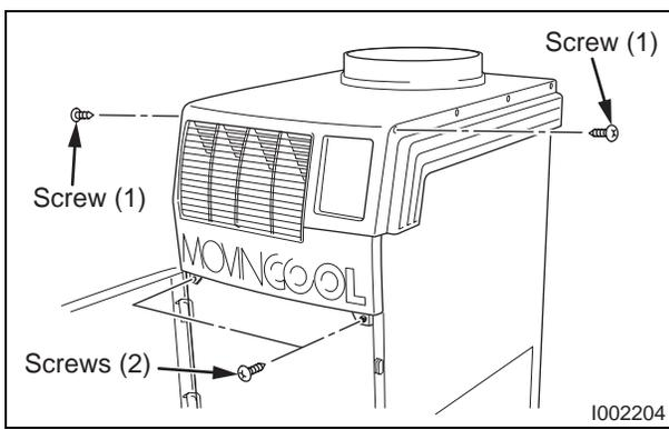
2) Remove four (4) screws from upper front panel.
