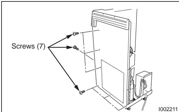
9) Remove seven (7) screws from right panel.
