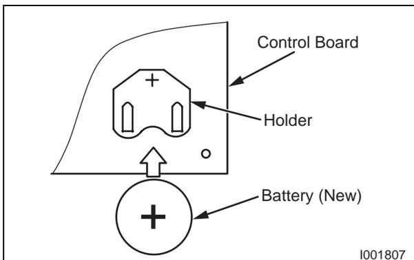
3) Insert new battery securely in the direction shown in the drawing.
