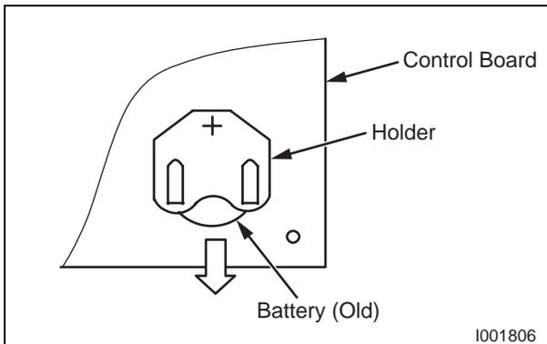
2) See diagram for battery removal.
