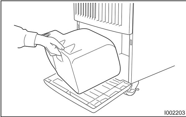
1) Remove drain tank.
