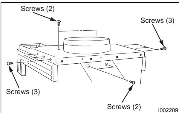
**7)** Remove eight (8) screws from rear panel and two (2) screws from blower housing (condenser).
