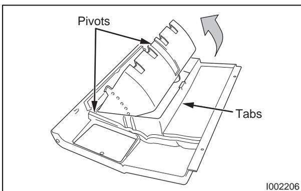
4) Louver can be removed from upper front panel by unsnapping the lock tap and removing the louver from its pivots.
