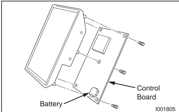
1) Disassemble control board. (See page 46 to 48.)
