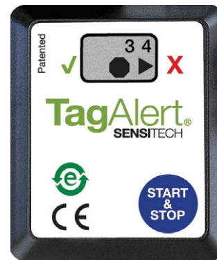
Holding Start & Stop button starts AlarmAlert mode, first displaying number of alarm, day of alarm, then timeframe alarm was triggered; This example shows alarm triggered day 7 of trip
